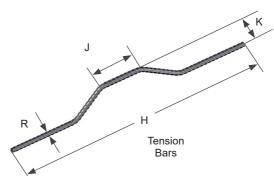
Note: FTB Tension Bars and FSV Shear Vees are made from Grade 60 reinforcing rod.
