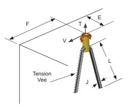
Note: Threaded Socket Anchor requires Tension Vee to develop tension capacity
